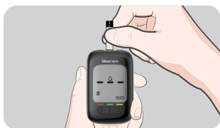
1 Insert Safe AQ Max II test strip
